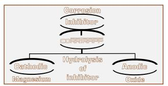
Anodic part of CORRTRAPP (Called corrosion and Passivation inhibitor) act by Reducing anodic reaction, that blocks the Anode Reaction and supports the natural reaction of passivation metal surface also due to the forming of film adsorbed on the metal. The inhibitor reacts with the corrosion product, initially formed, resulting in a cohesive and insoluble film on the metal surface.
